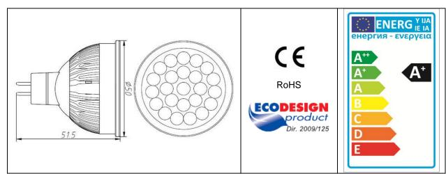
External Length =  $54^{\pm 2}$ mm; External Diameter =  $50^{\pm 1}$ mm
